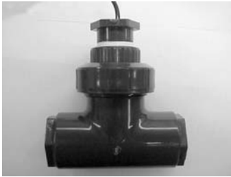
Model 399VP shown in Tee PN 915240-03, -04, or -05. Tee is available with 3/4 in., 1 in., or 1-1/2 in. NPT process connection threads.
