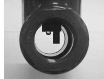
Side view of Tee PN 915240-03, -04, or -05 with Model 399VP shown in middle of process flow.
