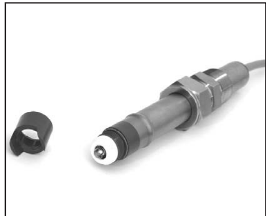
The metal process connector gives the sensor various insertions depths, depending on where the user locates the compression fitting. Also the threads can be switched to face the cable end of the sensor for connection to submersion pipes.
