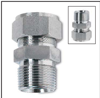
Metal Process Connector PN 23166-xx (xx = 00 for 316 SST and xx = 01 for Titanium) can be used for insertion or submersion connection to 1-inch tee fittings. It also must be used to connect Model 3400HT to ball valve PN 23240-00 or directly to the process.
