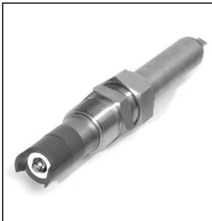
The metal process connector gives the sensor various insertions depths, depending on where the user locates the compression fitting. Also the threads can be switched to face the cable end of the sensor for connection to submersion pipes.
